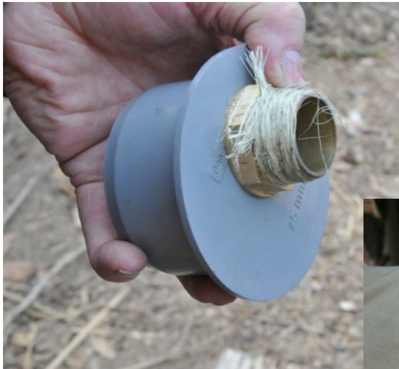
Detail of the fabrication and fitting: the completed drain valve for Type B
