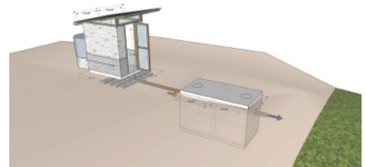
The current toilet and septic tank components
